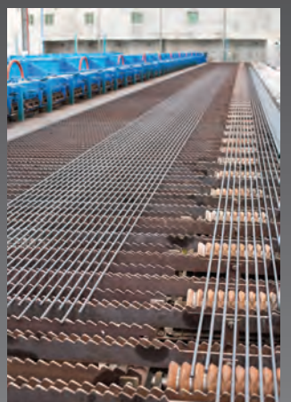
78 meter Cooling Bed
